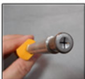
Place the NWDB or NWFB fastener onto the end of the tool
