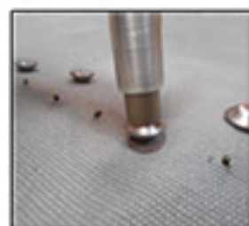
Using the tool, push the fastener down onto the cut shank
